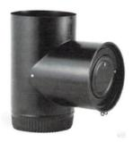
Read the manufacturers instructions for setting up your barometric damper. All Chubby Stoves require a turn damper in the pipe system (BEFORE) the barometric damper not (Above) it. This will keep your stove burning the same everyday and will stop overdrafting and excess coal consumption.
